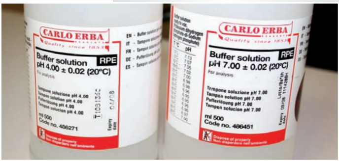
Buffers are used to calibrate the pH meter. © Dethioux
